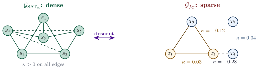
Figure 10: Fourier graphs \mathcal{G}_f for SAT_n versus a polynomial-size circuit. Left: the Fourier graph of SAT_n is dense and has strictly positive Ollivier–Ricci curvature on every edge (uniform green), because the rich cluster structure of Sol(F) forces many correlated high-degree Fourier monomials. The curvature-guided spectral descent (Definition 10.4) leaves this graph essentially unchanged (since curvature is already positive). Right: the Fourier graph of a polynomial-size circuit f_C is sparse (by the sunflower bound, Lemma 9.6), with most edges having near-zero or negative curvature (amber/blue). The descent drives negative-curvature components to zero (spectral excision, Definition 10.7), reducing \mathfrak{S}(f_C) monotonically to 2^{-\Omega(n)} (Lemma 10.8).
